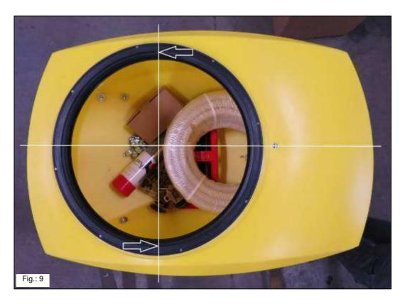
• Screw the hopper ring back on again with the previously loosened bolts. In doing so, ensure that the bolts are tightened with care.
