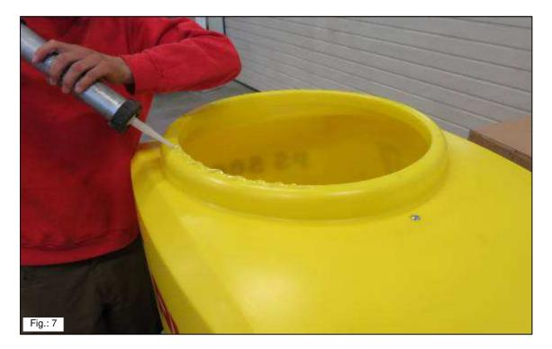
• After you have applied silicone to the entire circumference of the hopper upper edge (Fig.: 8), put the hopper ring back onto the hopper.
