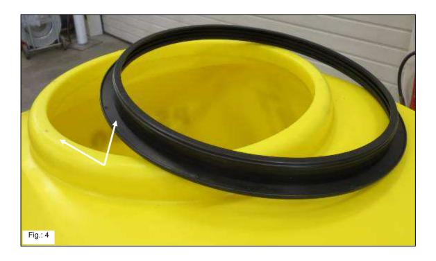
• In the next step, apply the enclosed bonding agent on both of these surfaces. To do so, use the enclosed brush (Fig.: 5, Fig.: 6).
