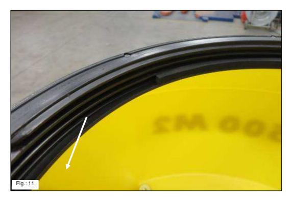
Now apply the enclosed sealing tape on the surface cleaned in the previous step on the inside of the ring.
